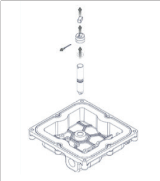
Figure 61. Removing the Shaft, Magnet & Magnet Holder
