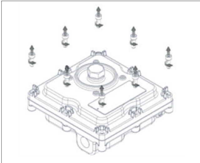
Figure 57. Remove the Cover of (KS + PTR) Series
