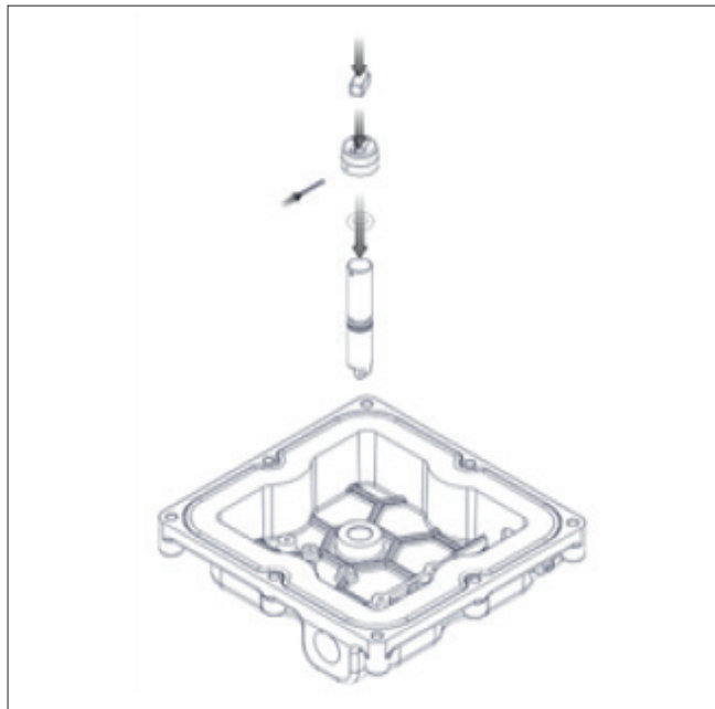
Figure 64. Inserting the Shaft Assembly on the Housing.
