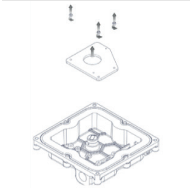
Figure 63. Removing Mounting plate.
