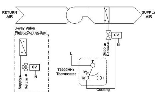
Cooling Only 2-pipe System with 3-speed Control Switch
