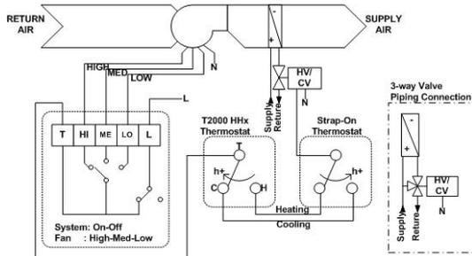
Heating & Cooling 4-pipe System with 3-speed Control Switch
