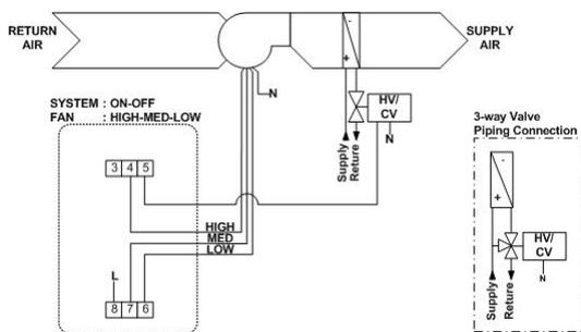
Heating/Cooling Only 2-pipe System with 3-speed Fan Control and Automatic Changeover
