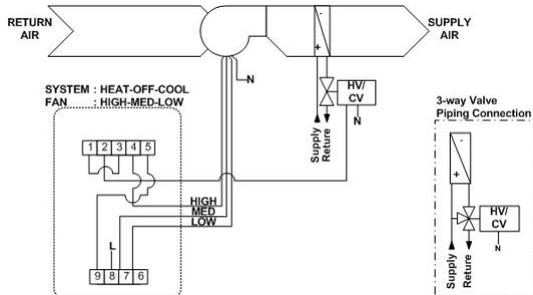
Heating & Cooling 4-pipe System with 3-speed Fan Control
