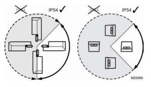
Fig 8. Mounting for IP54
