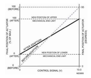
Fig 5. Adaption (function selection switch set to 0...10 V)
