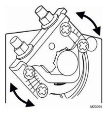
Fig 6. Mechanical end limits
