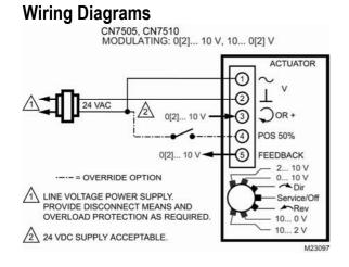
Fig 10. CN7505/CN7510 (modulating mode)
