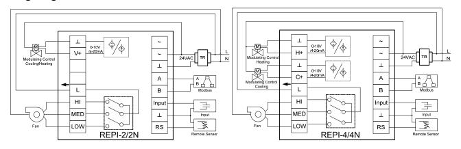
Note: Be sure to connect all the wires as per the wiring diagrams and keep it away from water, mud and other material so as to prevent the unit being spoiled!
